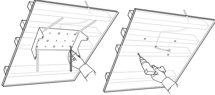
Minimum Installation Requirements when mounted to wood studs: 1 1/2" x 1/4" (38.1mm x 6.35mm) lag screw
