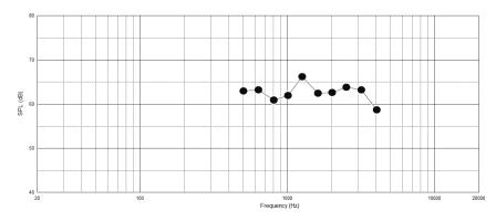
Contribution of each mid-range one-third-octave frequency band to the SPL (per EN54-24) when system is driven to Rated Maximum SPL (92 dB @ 4m; 101 dB @ 1m) using specified broadband pink-noise signal, 60W tap setting, 4m (Contribution figures: 500 Hz = 78.16 dB; 630 Hz = 78.59 dB; 800 Hz = 76.65 dB; 1000 Hz = 77.97 dB; 1250 Hz = 82.76 dB; 1600 Hz = 79.41 dB; 2000 Hz = 80.48 dB; 2500 Hz = 82.88 dB; 3150 Hz = 81.62 dB; 4000 Hz = 76.67 dB).
